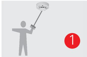
Press the user key for **1 second** (e.g. using a broom handle as an aid).
