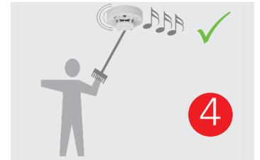
Press the user key for approx. **5 seconds**. If the **test alarm** sounds (1 sec. on / 1 sec. off), the **smoke alarm is in working order**.
